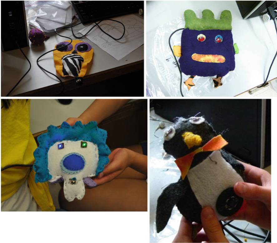
Fig. 14.4 Sample student Plushbot projects. Upper left : an owl figure. Upper right : an alien that senses temperature changes and uses an LED light to indicate the change. Bottom left : a lion with flashing LED eyes. Bottom right : a penguin that responds to light changes by singing a song and flashing an LED light
